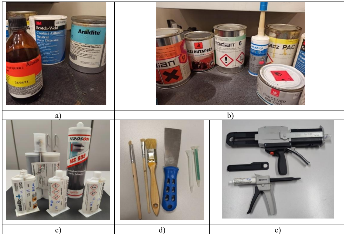
Figure 3 – Examples of substances and necessary equipment for gluing (stage II): a) primers, b) adhesives for mixing, c) adhesives in tubes, d) brushes, putty knives, tips for glue application, e) devices for squeezing two-component adhesives
